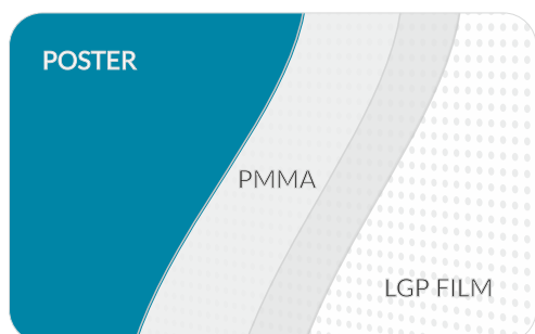
Cross-section of the backlight unit
