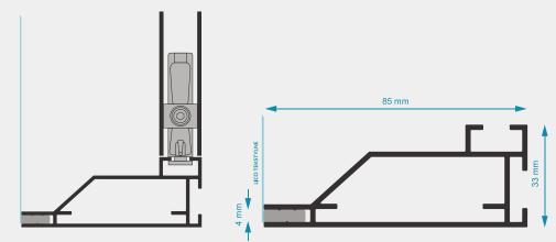
Despite the light construction, the frame is additionally stiffened with internal connectors made of aluminum, which additionally prevents the so-called "light escape" through the corner edge of extrusions.
