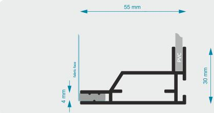
Despite the light construction, the frame is additionally stiffened with internal connectors made of aluminum, which additionally prevents the so-called "light escape" through the corner edge of extrusions.
