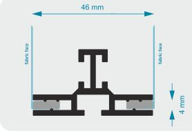
Despite the small width, just 46 mm, the lightbox is sufficiently stiff due to the use of two steel connectors placed in grooves in the central part of the extrusion.
