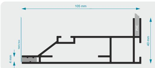
Lightbox frame is additionally stiffened with internal connectors made of aluminum, which additionally prevents the so-called "light escape" through the corner edge of extrusions.
