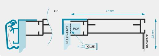
The angle extrusion marked at the drawing creates an aesthetic, uniform surface with the side of the lightbox.
