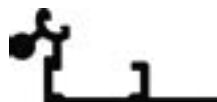
137124 Basisprofiel 32/45 mm zonder nok Basic profile 32/45 mm without ridge Basisprofil 32/45 mm ohne Nocken
